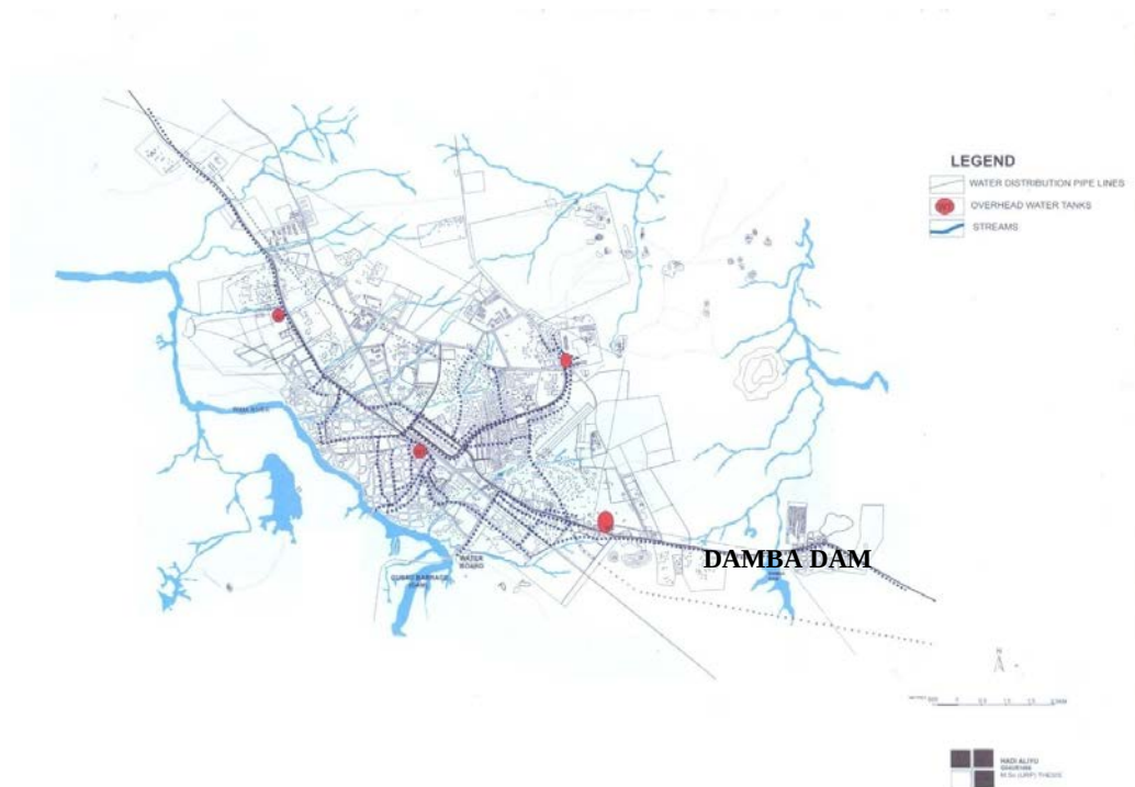
Fig.3 Water Distribution Facilities in Gusau
